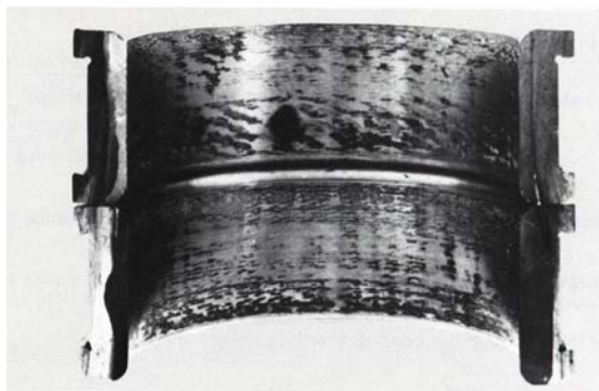
Figure 2.12 Fretting corrosion (FAG, 1985).
