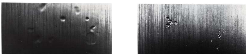
Figure 2.8 Indentation due to hard particles (FAG, 1985).
