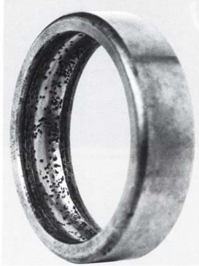
Figure 2.10 Corrosion due to rust (FAG, 1985).
