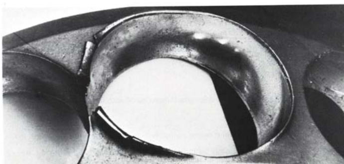
Figure 2.28 Cage fracture due to misalignment (FAG, 1985).
