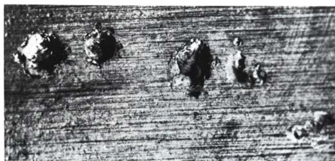
Figure 2.15 Craters due to arching in a cylindrical roller bearing (FAG, 1985).
