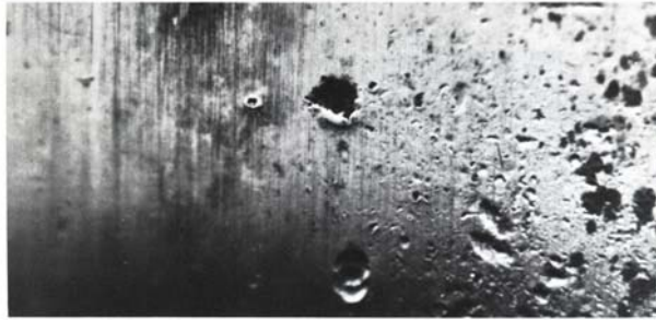
Figure 2.9 Indentation of brittle particles (FAG, 1985).
