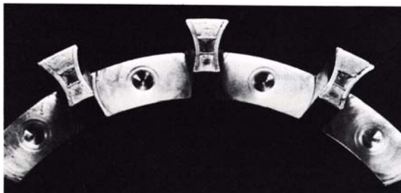
Figure 2.27 Cage fracture due to vibration (FAG, 1985).
