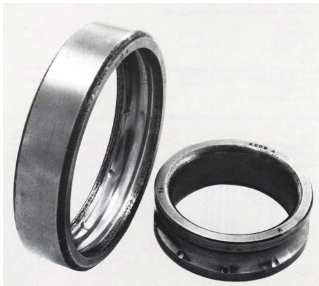
Figure 2.7 Indentation of soft particles (FAG, 1985).
