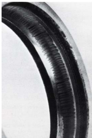
Figure 2.14 Fluting in the outer ring raceway of a deep groove ball bearing (FAG, 1985).
