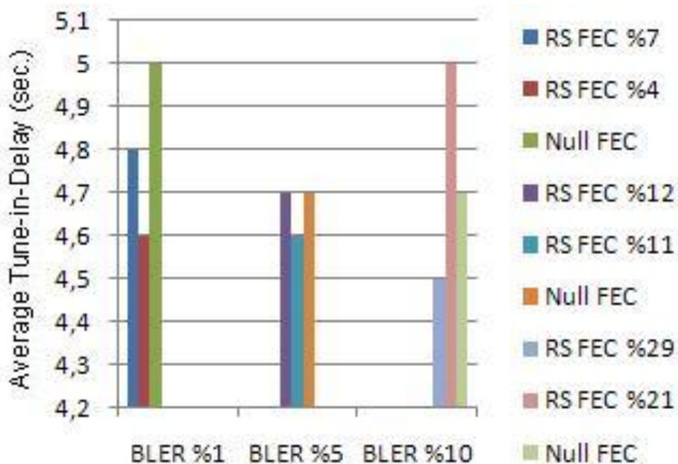
Figure 13.5 Average tune-in-delay results according to selected FEC overhead ratio with respect to bearer rate 256 kbit/s and BLER 1,5, 10%.
