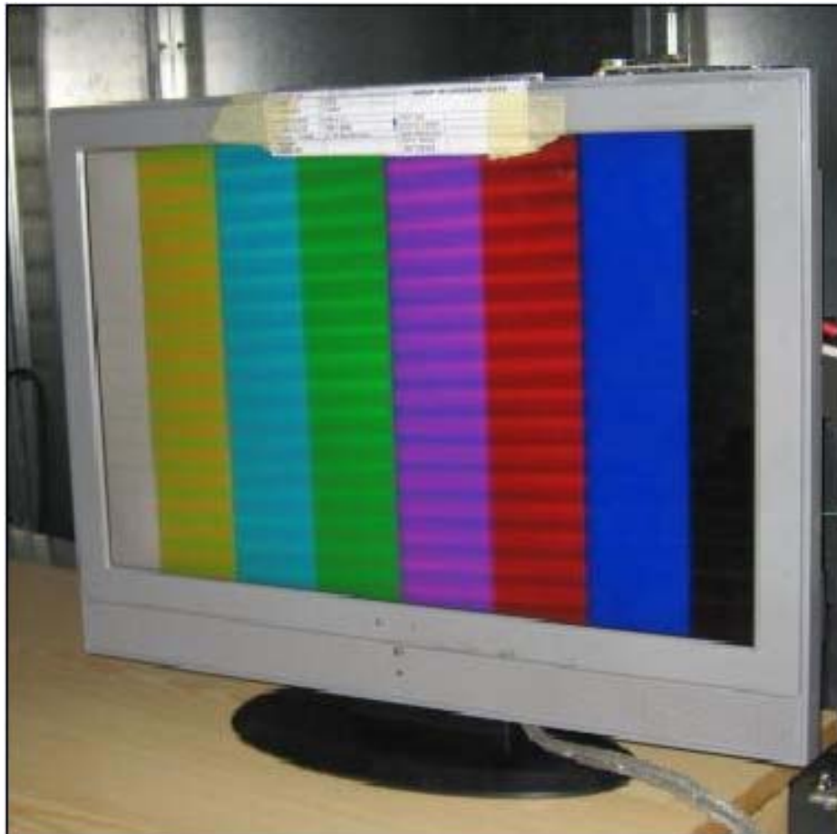
Figure 5.3 The degradation of the picture during S2c test
