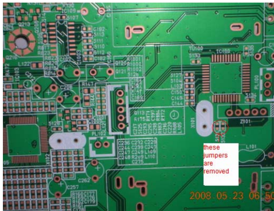
Figure 5.14 The jumpers removed to increase immunity
