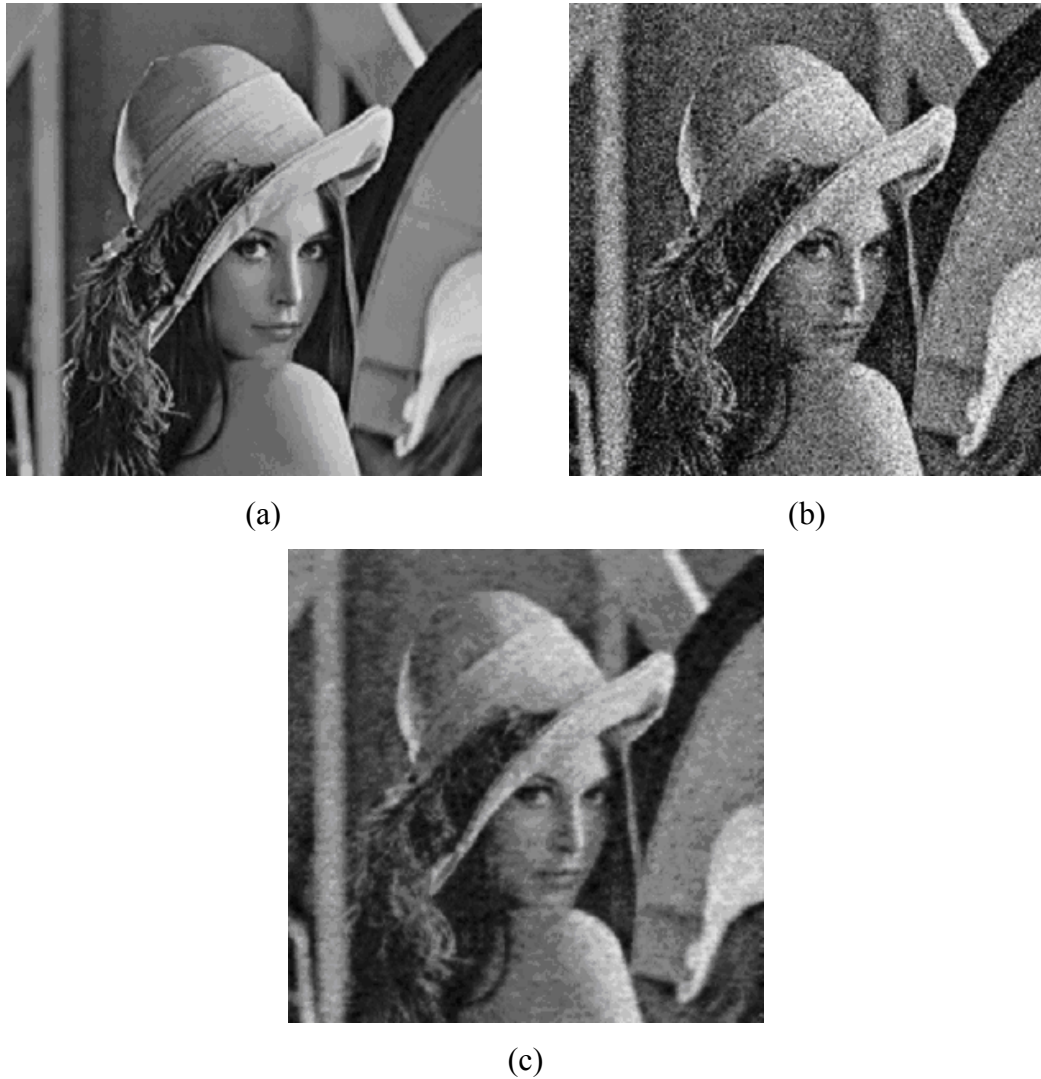
Figure 4.3 (a) Original Lena image, (b) Noisy image (PSNR = 20.269dB, SNR = 6.5669), (c) Filtered image (Block size = 1x1).
