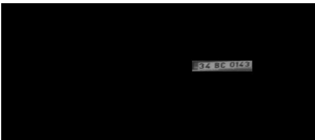
Figure 4.23 Result of performing plate extraction.
