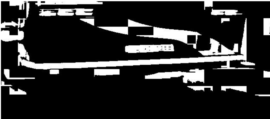
Figure 4.27 Result of performing smearing algorithm on thresholded image.
