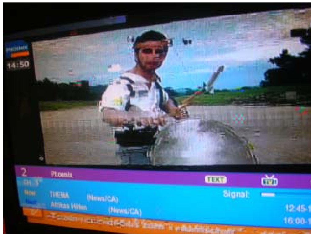
Figure 4.23 Digital blocking problem and signal level.
