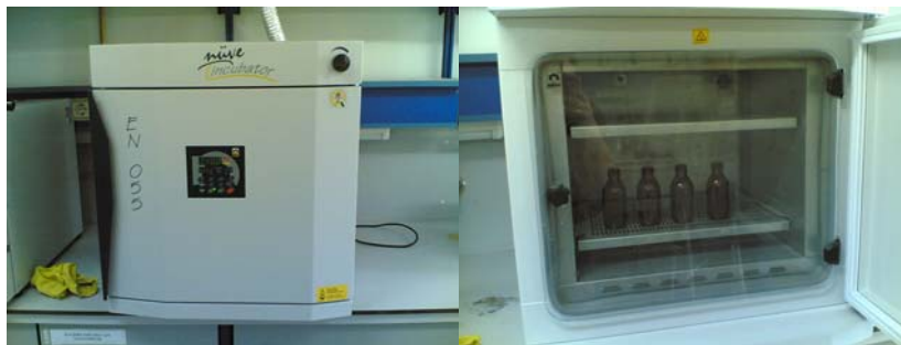
Figure 3.5 Incubator used for BMP test
