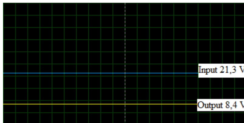
Figure 4.11 Simulation result of buck converter for red leds, y=5V/div
