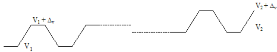
Figure 2.13 If larger output capacitance is used, it takes the charge pump longer to reach its steady state.
