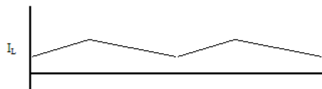
Figure 2.40 Forward converter L current
