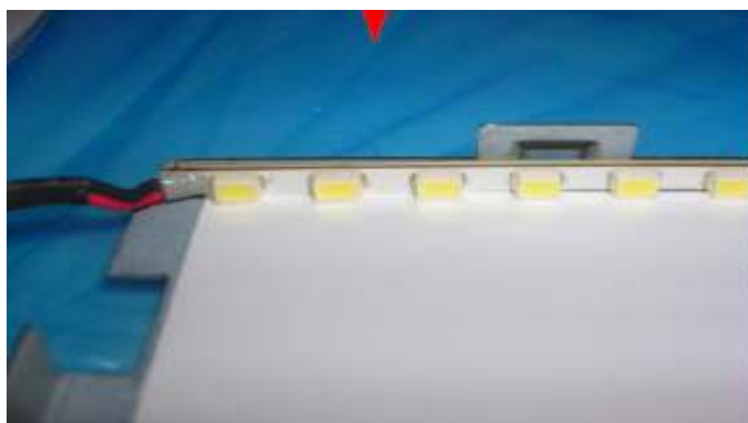
Figure 2.6 Edge Lit type backlight
