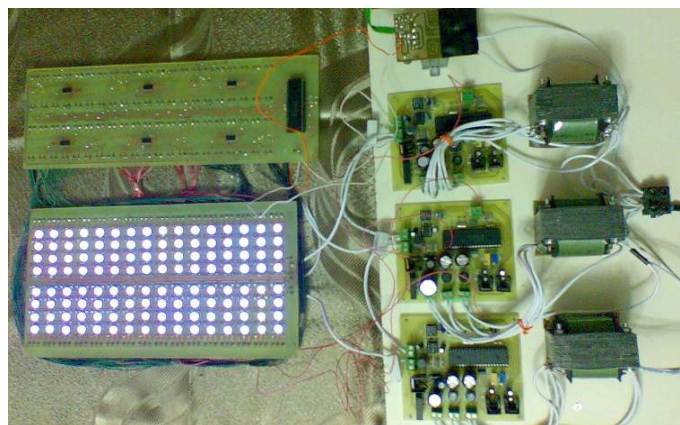
Figure 4.31 Full circuit when all leds are lighting
