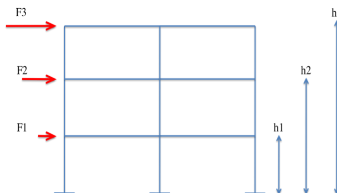
Figure 4.20 Applying the static load at each storey.
