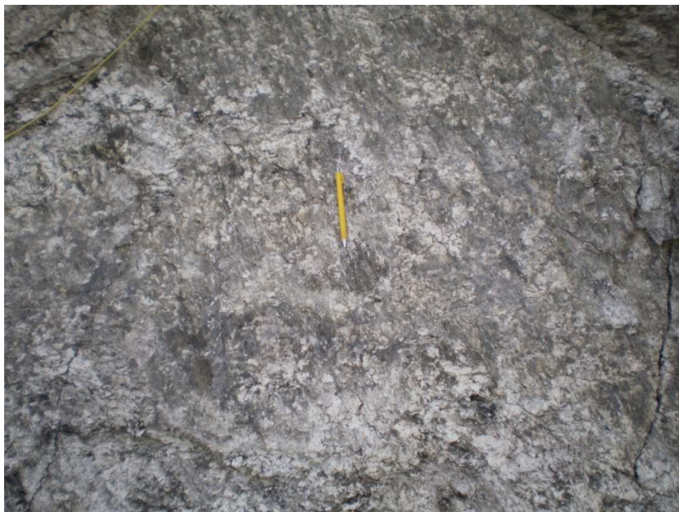
Figure 6.2 The view of slickensided and undulating foliation plane.
