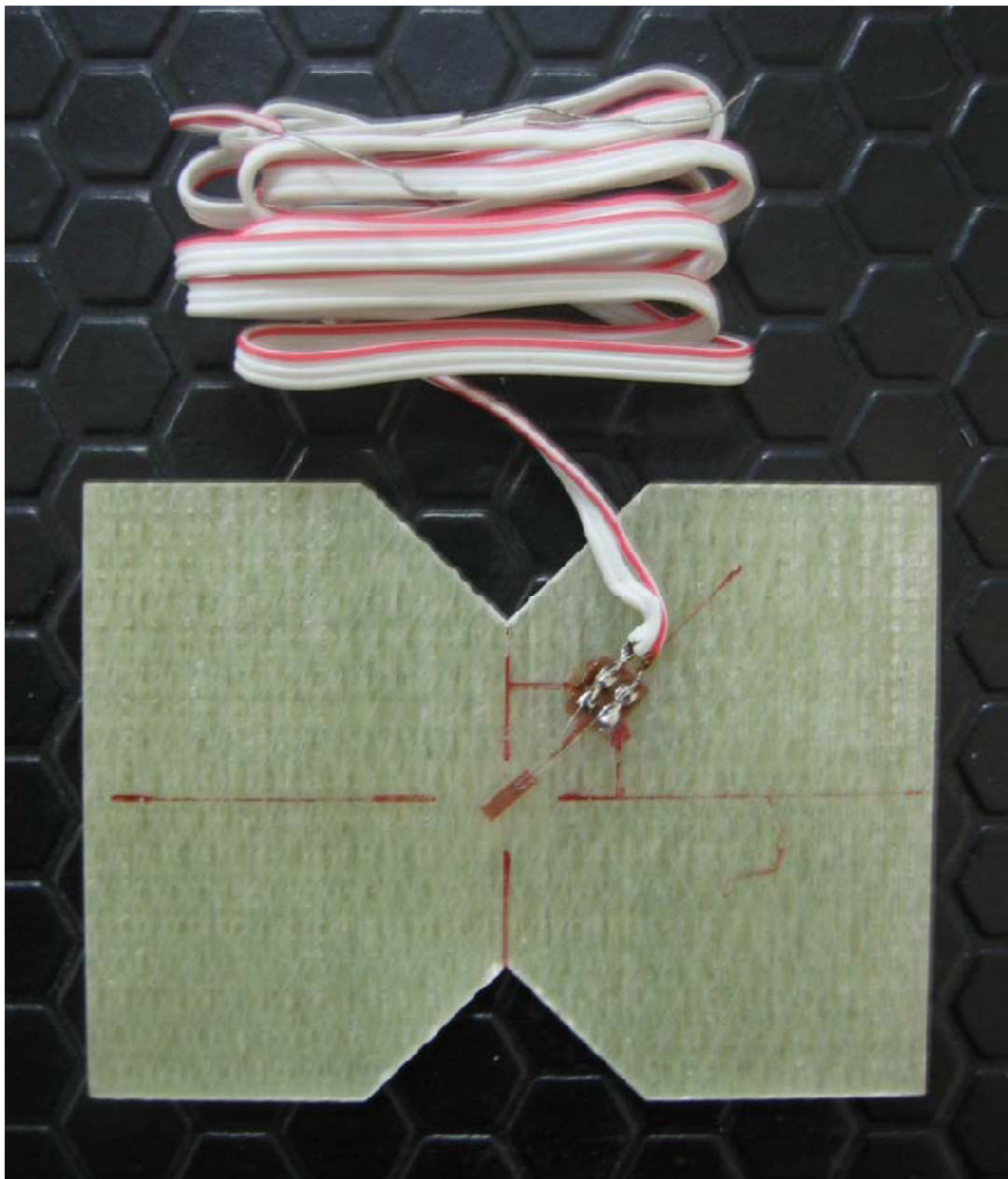
Figure 3.11 V-notched rail shear test specimen before tested.
