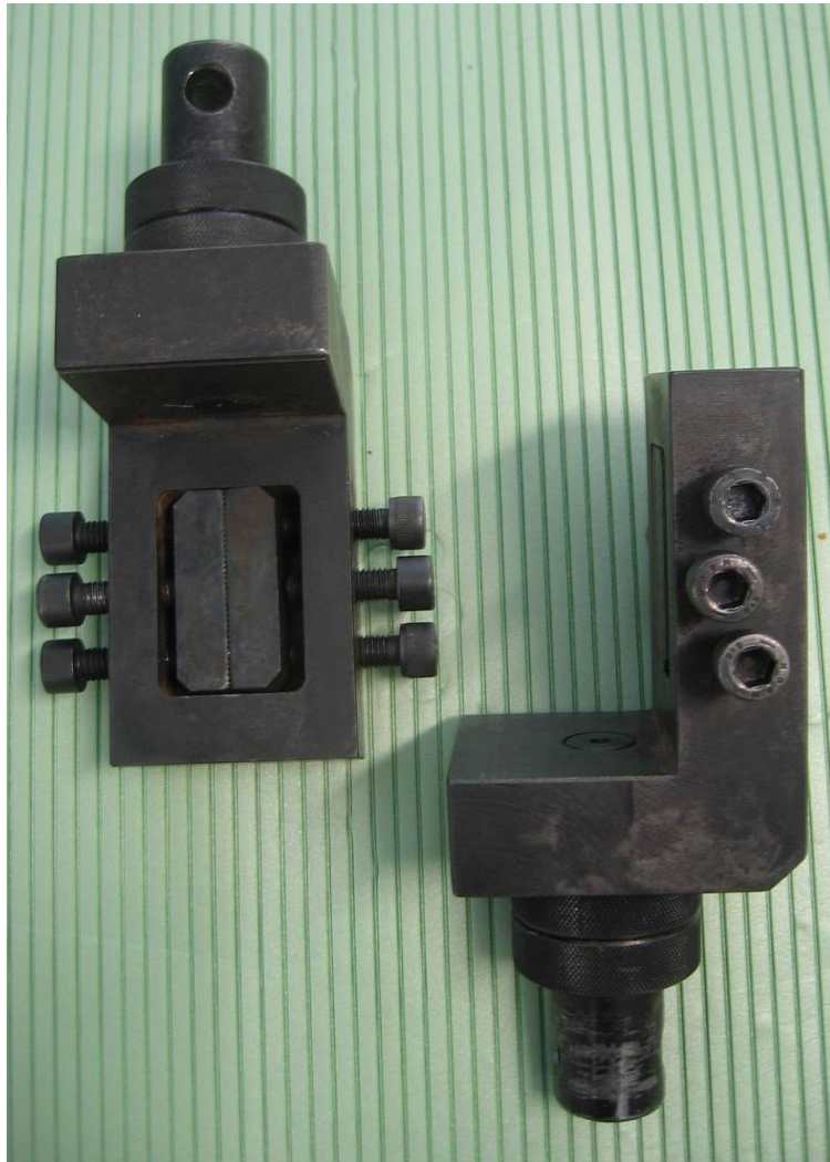
Figure 3.10 V-notched rail shear test equipment
