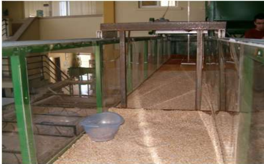
Figure 5.14 System to make a fix bed level. ( Bombar, 2009)
