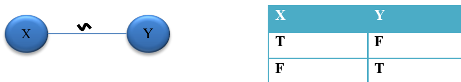
Figure 6.6 The notation and truth table of negation operator
