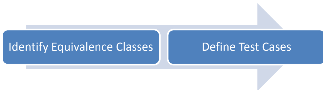
Figure 5.2 Steps of equivalence partitioning software test case technique
