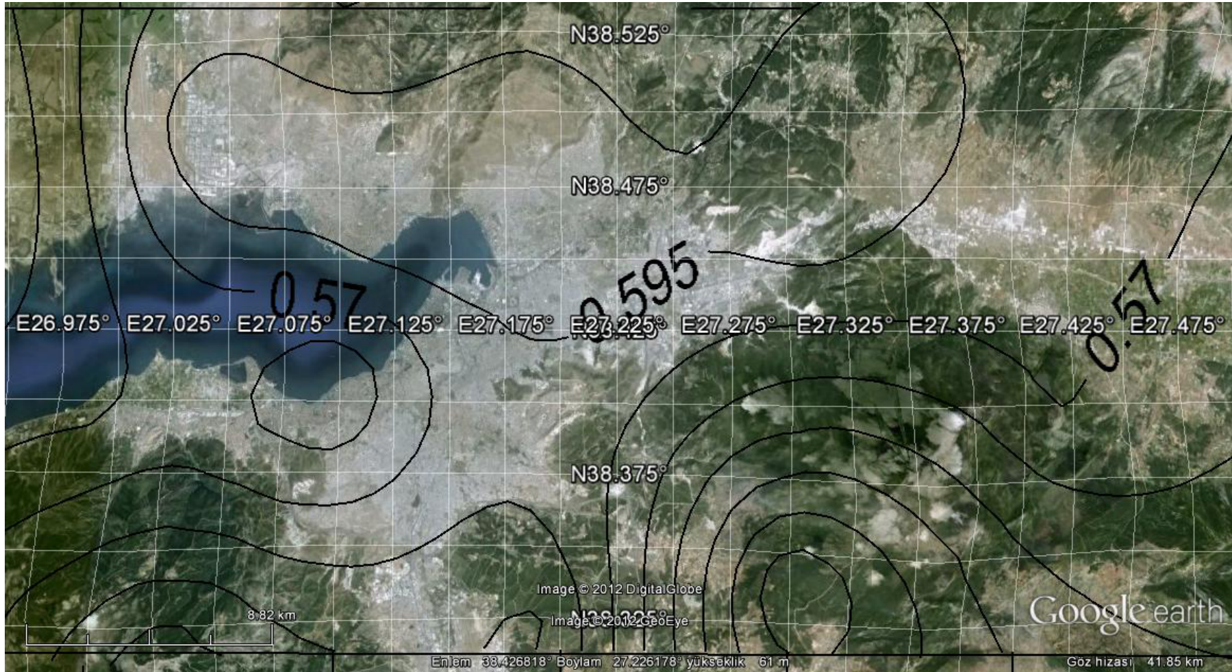
Figure E.29 (MAP 29): Attenuation relationship: Boore & Atkinson (2007). Probability of exceedance in 50 years: 10% Values: Ground Acceleration (g) (Median) Spectral period T=0.2 s V_{s30}=760 m/s
