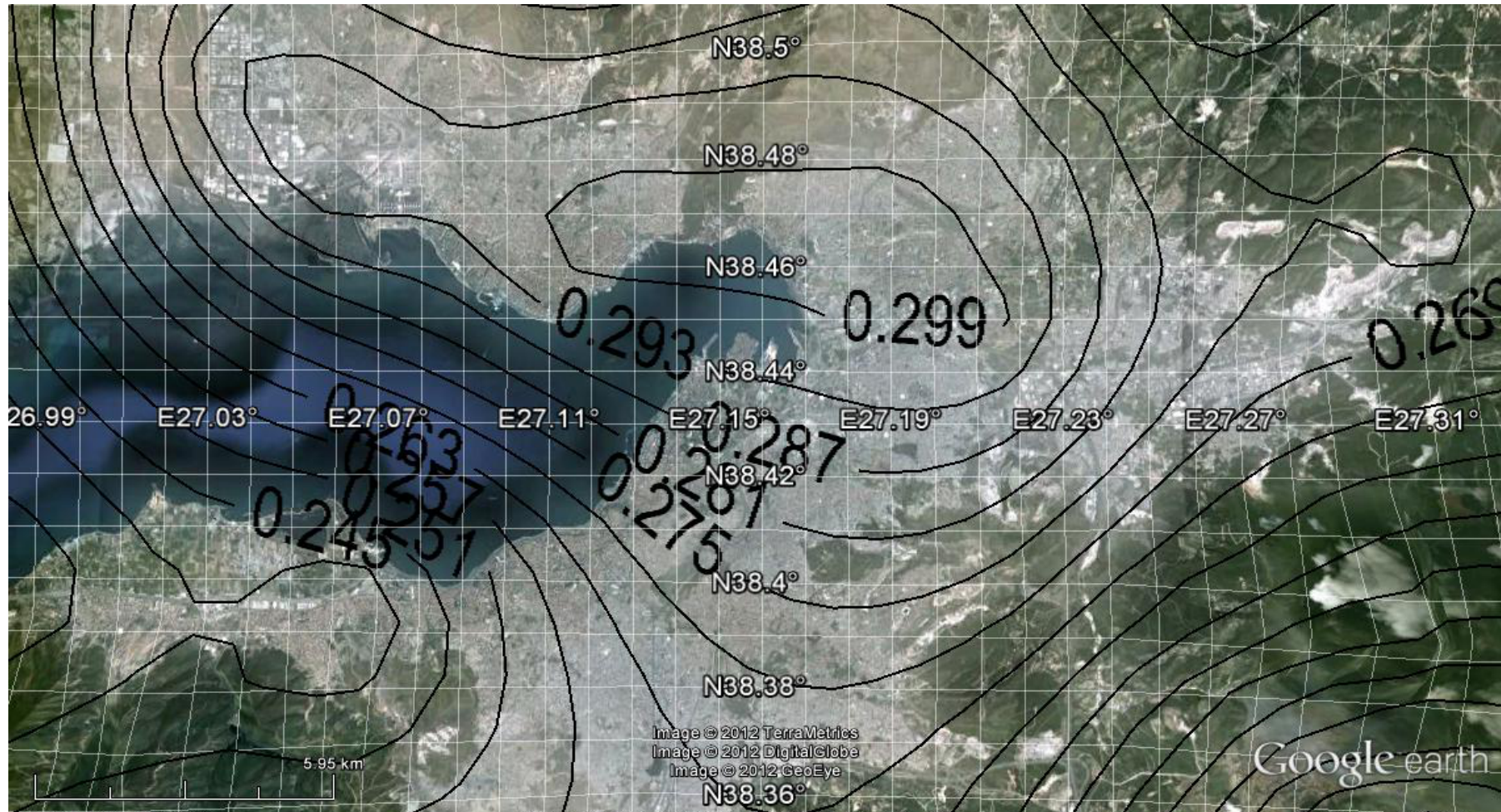
Figure E.14 (MAP 14): Attenuation relationship: Brian et al. (2008). Probability of exceedance in 50 years: 10% Ground Acceleration (g) (Median) Spectral period T=1 s V_{s30}=760 m/s
