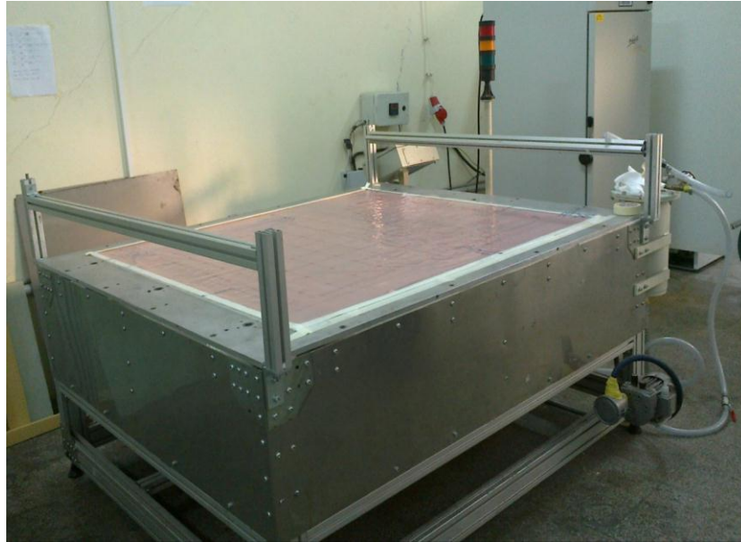
Figure 3.2 A photo of vacuum assisted resin infusion molding (VARIM) equipment
