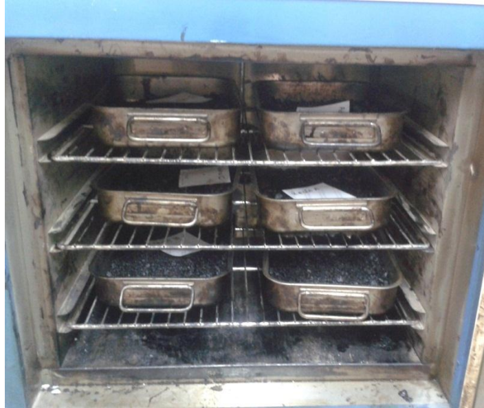
Figure 4.14 Short-term conditioning in a forced-draft oven set for 135°C for 4 hours
