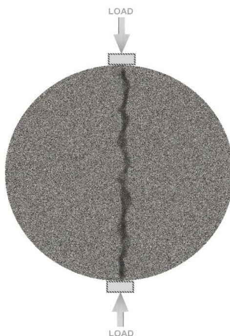
Figure 4.16 A possible crack pattern for IDT test
