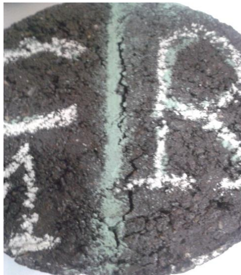
Figure 18 A cracked specimen after IDT test
