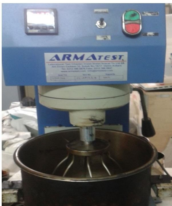
Figure 4.12 Mixer used in mixing of the aggregates and the bitumen
