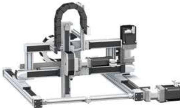
Figure 2.4 Cartesian robot (Lexium MAX, Schneider Electric)
