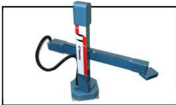
Figure2.5 Cylindricalrobot(R19 ATHENA series, ST ROBOTICS)
