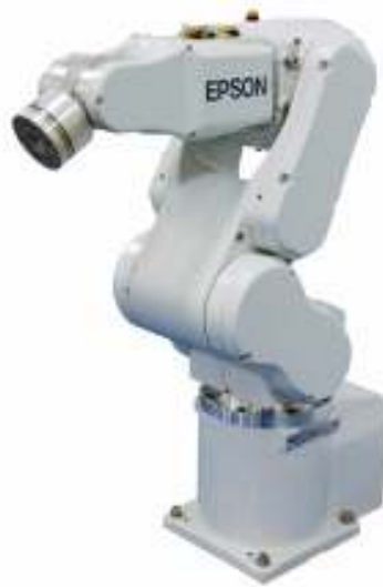
Figure 2.3 Articulated robot (C3 Series, Epson)
