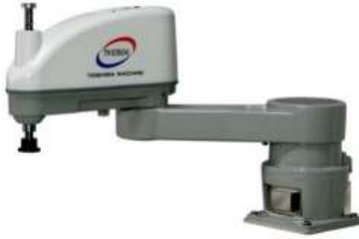
Figure 2.2 Scararobot (Toshiba Machine TH650 A)
