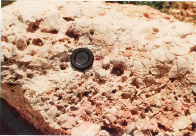
Figure 3.18 Consolidated Conglomerates Composing of Limestone Clasts that Cemented Carbonate Matrix. The Scale is 5 cm in Diameter.
