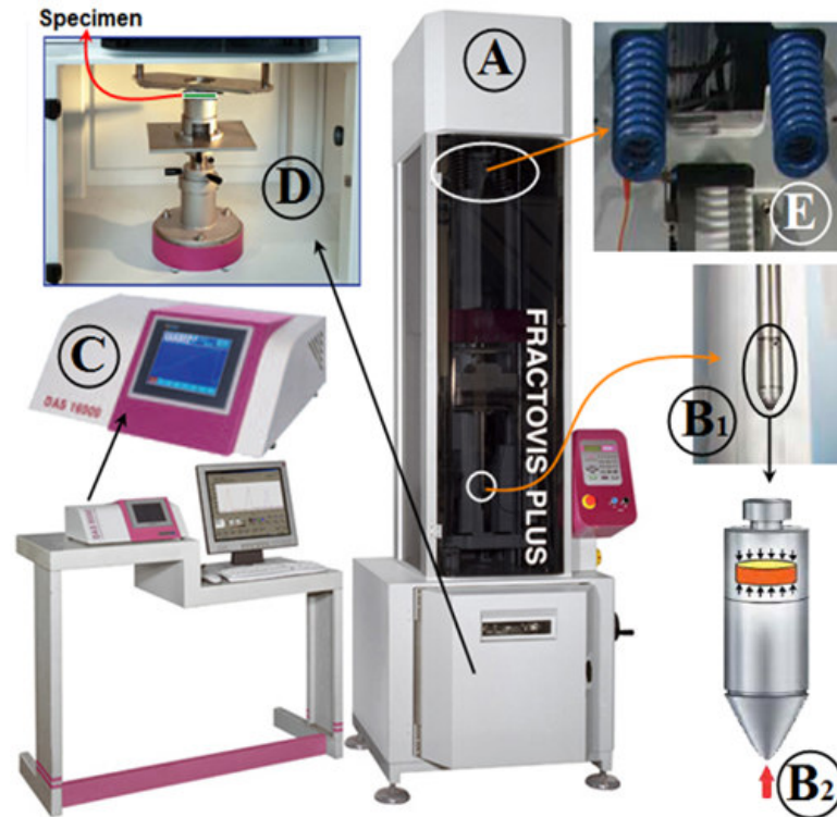
Figure 5.1 Fractovis Plus Low velocity impact tester (A) and its equipments; impactor nose (B 1 ), piezoelectric impactor nose (B 2 ), Data Acquisition System (DAS) (C), the specimen clamp mechanism (D), and the springs (E).
