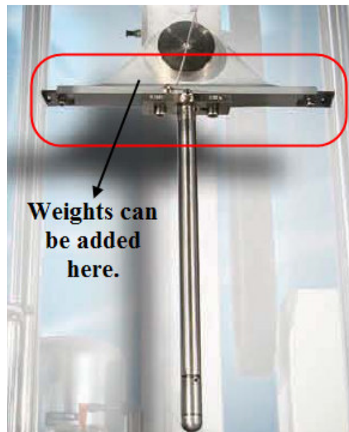
Figure 5.4 Weight adding unit.
