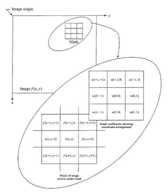
Figure 4.4 The mechanics of spatial filtering
