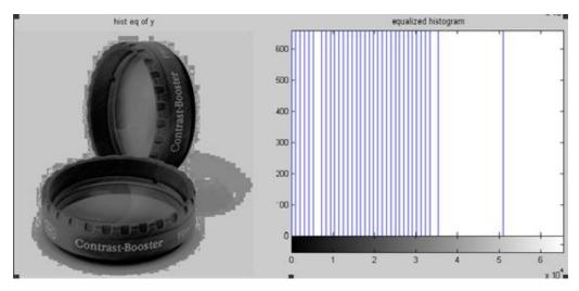
Figure 3.3 Standard HE applied to image and its histogram with "histeq" command
